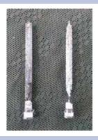
Hot water system anode on left is from an RV using the DELTA RV for 12 months. compared to anode on RV with no DELTA treatment. See full story overleaf.
